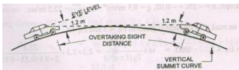
Figure: Measurement of overtaking sight distance
