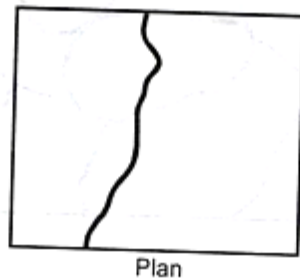
Longitudinal cracking due to differential volume change
