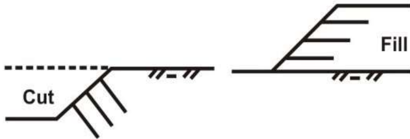
(c) Reinforced cut and fill slopes
