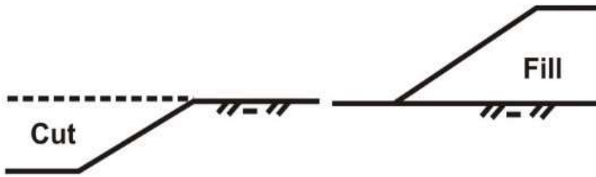
(a) Unreinforced cut and fill slopes
