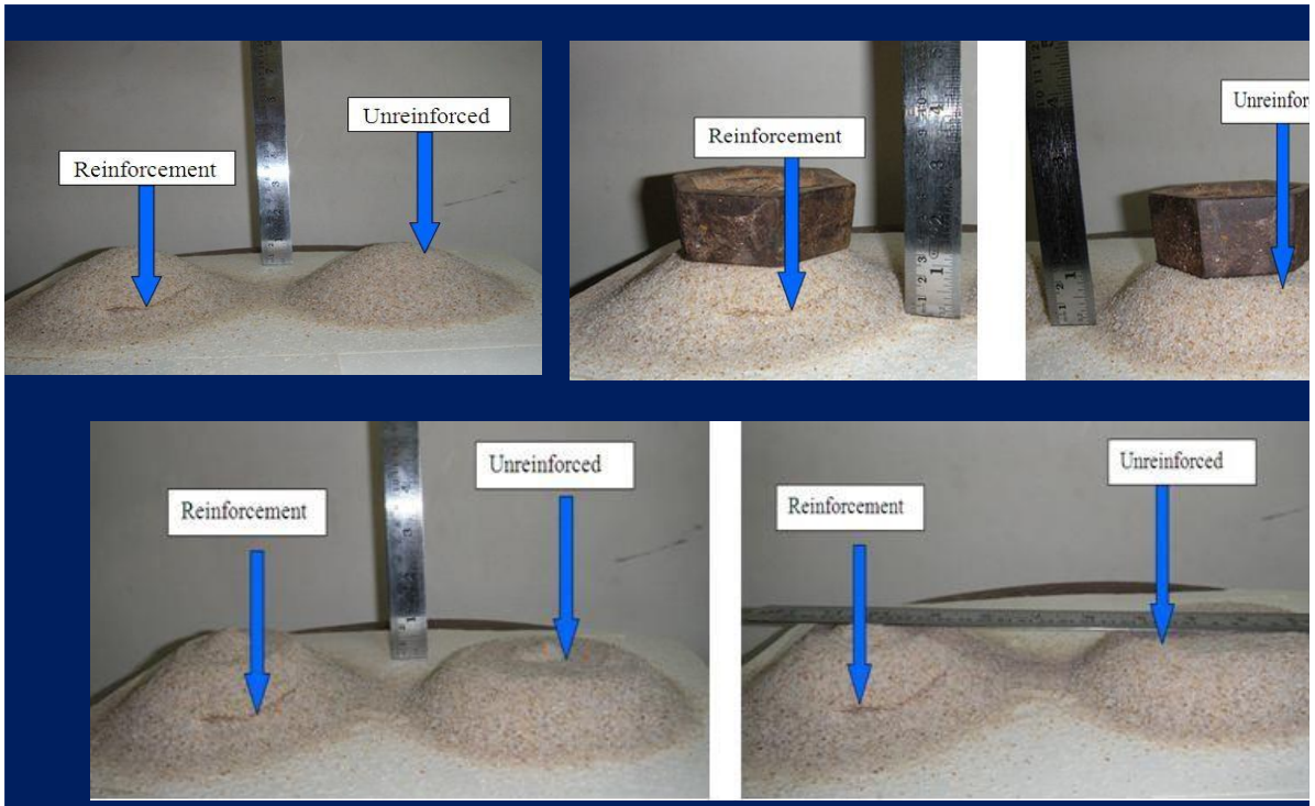
Figure 4 Difference in slope and settlement after loading
