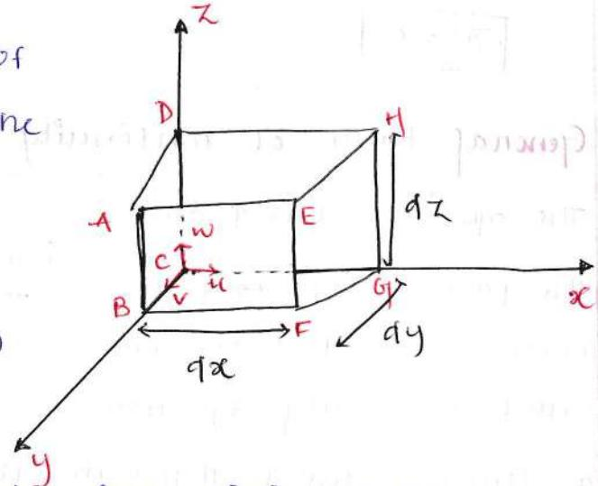
since the mass is neither created nor destroyed in the fluid element, the net increase of mass per unit time in the fluid element must be equal to the rate of increase of mass of fluid in the element. But mass of fluid in the element is  $\rho, dx dy dz$  and its rate of increase with time is  $\frac{\partial}{\partial t}(\rho, dx dy dz)$  or  $\frac{\partial \rho}{\partial t}, dx dy dz$ .
