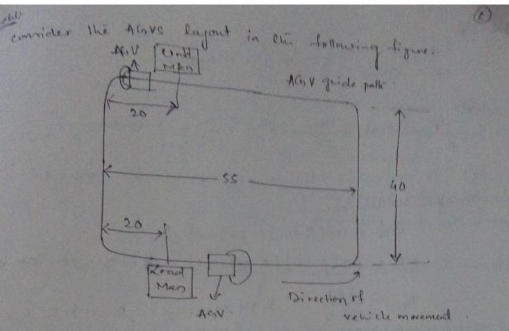
The vehicle travel counter clockwise around the loops du deliver leads from the lead stations to the coload station. doading time at the load station = 0.35 min and unloading time at the coload station = 0.50 min. How many vehicles are required to satisfy demand for this largood if a total of 40 del/mr. must be completed by the AGVS.
