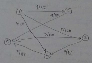
Nodex represent the load/unload stations and arrows. are lebeled with flow rates and distancex.
