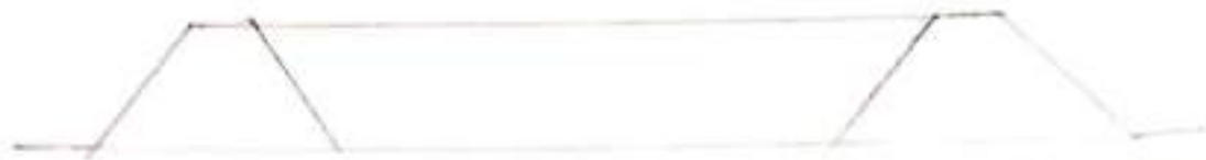
Above Ground landfill with Embankments
