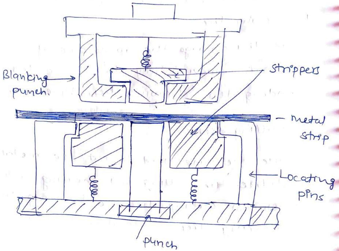
In these dies washer is produced by simultaneous blanking and piercing operation.
