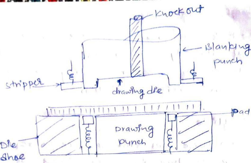
A drawing punch of required shape is fastened to the die shoe. The blanking punch is attached to punch holder. A spring stripper strips the skeleton from blanking punch.
