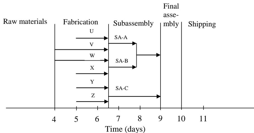
The chart shows that part V & W started on 4<sup>th</sup> day and the other parts on 5<sup>th</sup> day such that all the components become ready for subassembly on 6.5<sup>th</sup> day and all the subassembly become ready on 9<sup>th</sup> day for final assembly. The assembly is over on 10<sup>th</sup> day.
