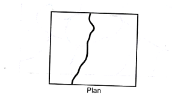
Longitudinal cracking due to differential volume change
