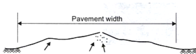
Failure due to frost heave
